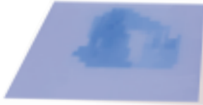
Actual test film showing instant real-time result of dosimetry
