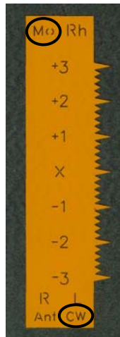
Figure 2. Labeling of film strip to identify anode track and field edge. Film strip labeled for chest wall edge of Mo track.
